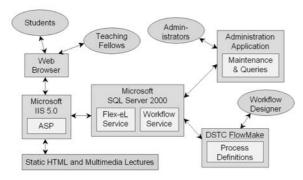
Figure 1. Flex-eL Technology Architecture
